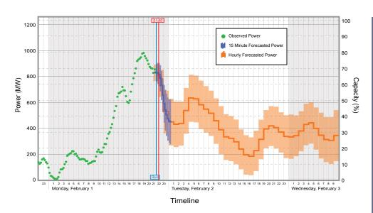
Many power systems with relatively high shares of wind power have integrated wind forecasting into system operations. This graphic, based on sample wind forecasting output for Xcel Energy (a utility in the United States), shows a wind power forecast over a 36-hour horizon, including actual power generation (green dots) up to the initial forecast point, the predicted wind power (solid line), and the typical forecast error from the preceding seven days (shaded area) [1].
